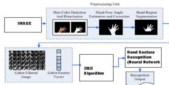
Figure 2. Hand Gesture Recognition Process
