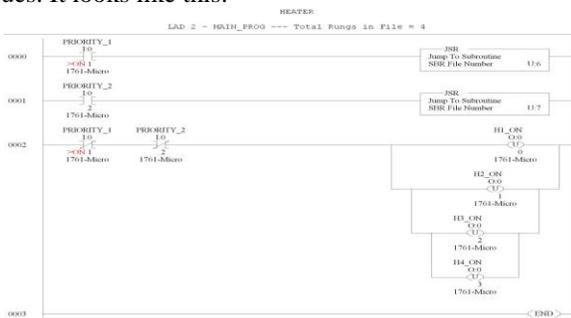
Figure 1: A part of Ladder Logic for heater control.
