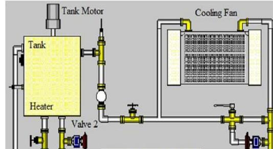
**Figure 3: SCADA diagram for the system.**
