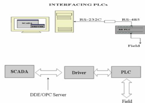
**Figure 4: Interface diagram of PC to PLC and to SCADA.**
