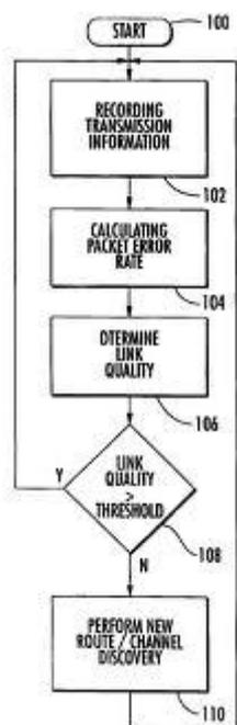
Fig.8- working steps diagram on AODV
