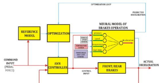
Figure 1: Intelligent control of automotive braking system
