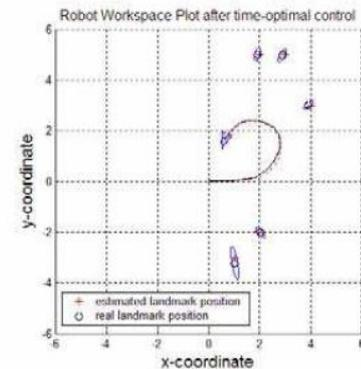
Figure 4. The SLAM results at the completion of the time-optimal control
