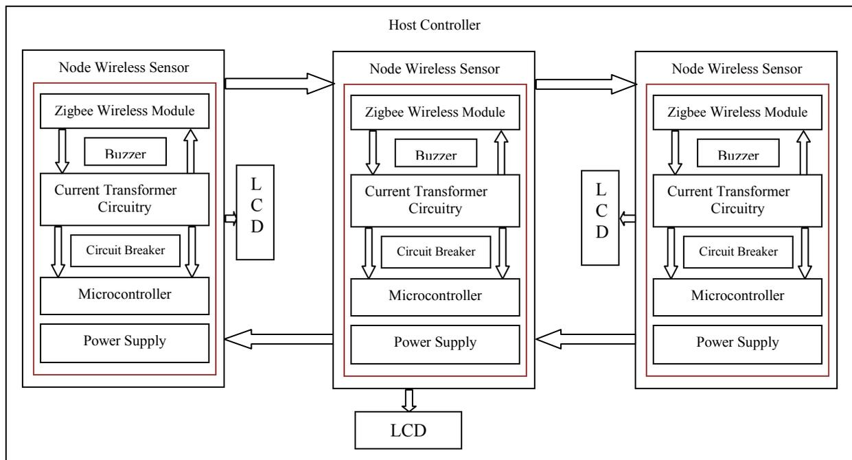
Figure 2. Block diagram of Power theft monitoring system
