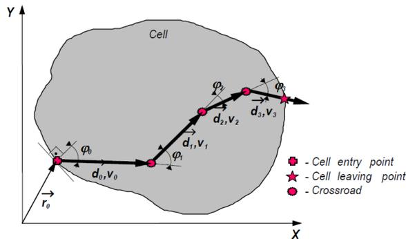
Fig2. Tracing a mobile within cell
