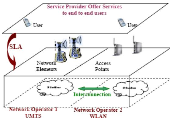
Fig.1. Architecture of Heterogeneous Network
